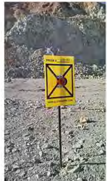
A typical prism with back target. Used with survey and 3D point monitoring systems to measure changes in elevation and position of a point.
