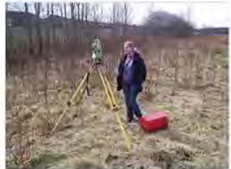
Archaeological survey using a Leica TPS1100 total station on an Iron Age dwelling in Ytterby, Sweden
